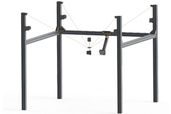
**Fig. 1.** Construction of an underconstrained, cable-suspended parallel manipulator with four cables for spatial positioning of an end-effector using gravity.
