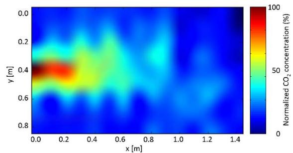
**Fig. 2.** Bilinear interpolation of the gas distribution measured by the robot's payload during experiments. Air flow from left to right with source located at the left mid-section.
