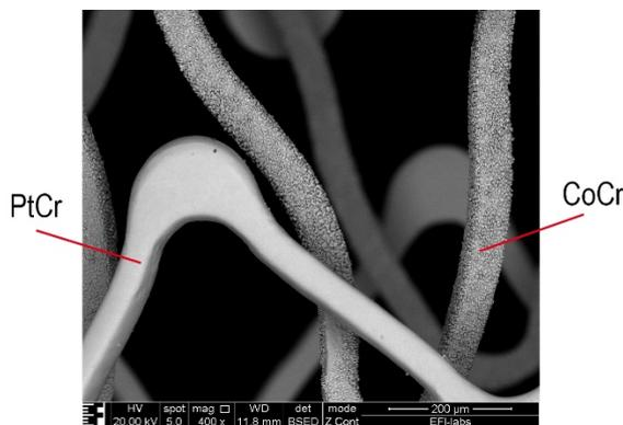
**Fig. 2.** SEM image of the stents after 1+1 hour of corrosion test
