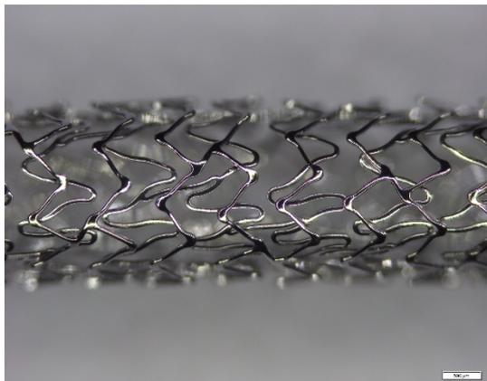
**Fig. 1.** Stereomicroscopic image of the overlapping stents, CoCr stent is surrounded by the PtCr stent
