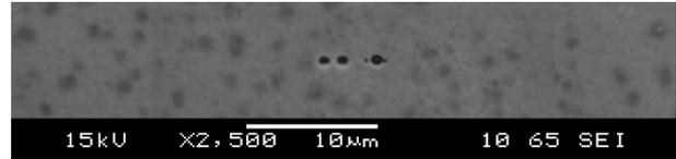
**Fig. 3.** Pitting corrosion on the PtCr stent
