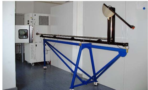
Fig. 1. Hopkinson Bar with its front end integrated in a temperature chamber.
