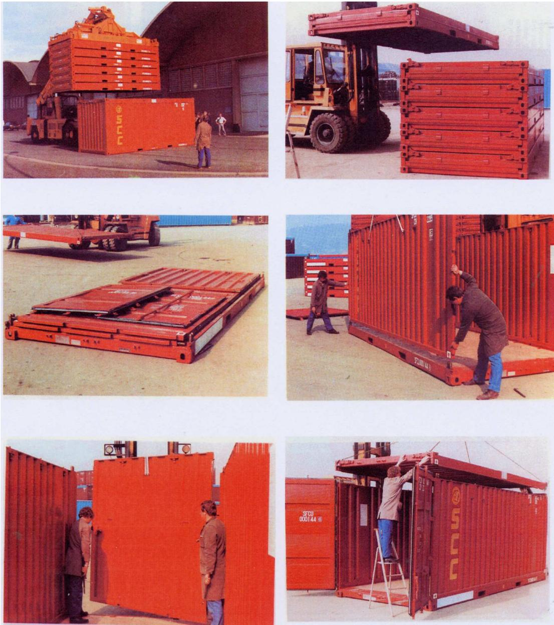
Fig. 2. The folding process of the Six-in-One container
