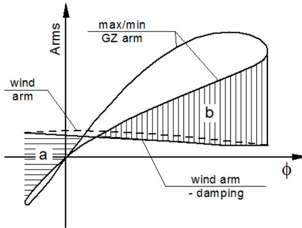
Fig 2. Diagram illustrating the application of the Energy Balance method.
