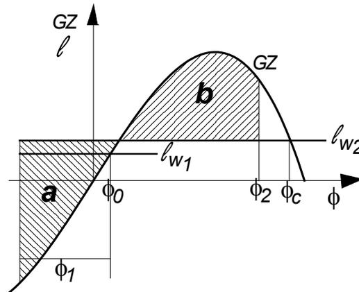
Fig 1. Diagram illustrating the application of the Weather Criterion.
