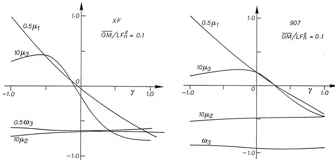
Fig 5. Variations of the eigenvalues of the characteristic equation corresponding to the system of differential equations of anti-symmetric motions as a function of trim for two hulls of BSRA series. Model XF (left) with B/T=1.907 and 907 (right) with B/T=3.437 [36].
