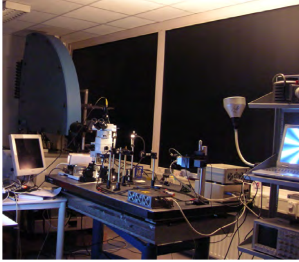
Figure 5.3 Picture of the combined Brandaris camera and optical tweezers setup (Feb 03, 2006)
