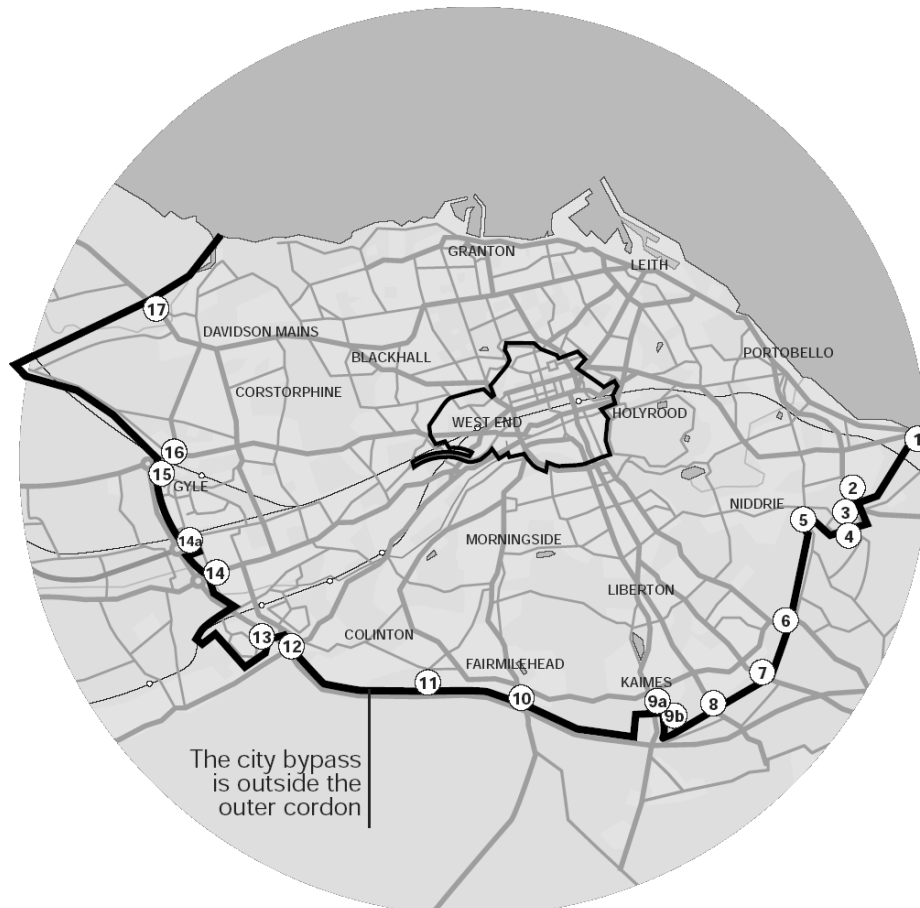
Figure 1: Map of Edinburgh showing the network of major roads (grey) and the location of the proposed inner and outer charging cordons (black). The numbered circles show the location of charging entry points in the outer cordon. The diameter of the mapped area is approximately 16 km (adapted from CEC, 2004b).
