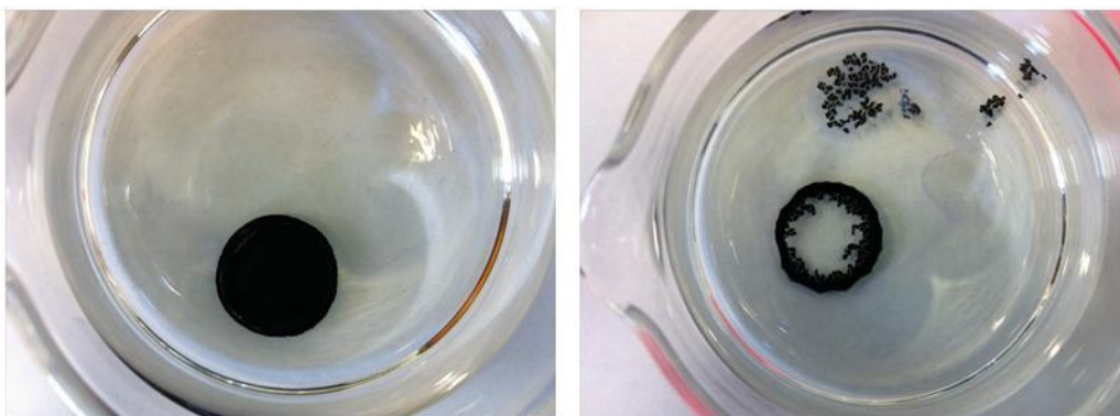
Figure 22. Chitosan/CNTs membrane with positively charged f_1 -CNTs (left) and pristine CNTs (right) dipped in acetone during the degradation process of the filter.
