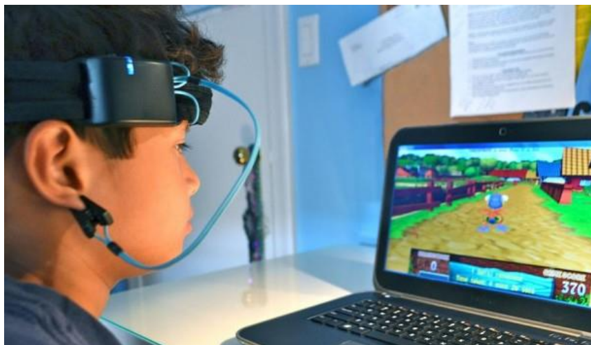
Fig. 1m: a young user experiencing a BCI-mediated NF treatment based on the voluntary modulation of attention-related brainwaves (neurogadget.com)
