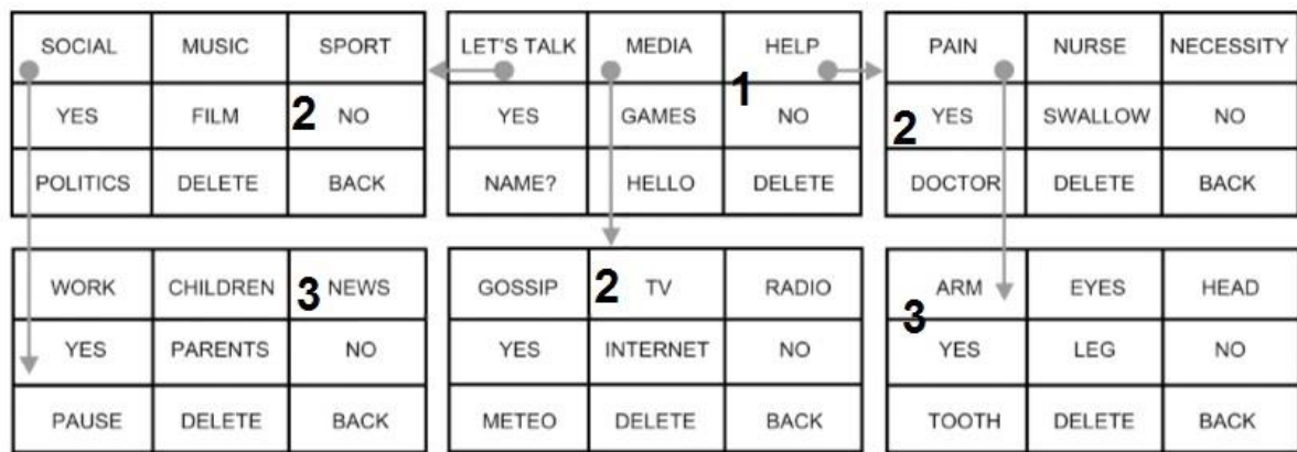
Fig. 2.1a: Multimenu structure (modified version of an original figure contained in Jarmolowska et al., 2013). The main menu (1) allows to communicate direct, fast sentence or to enter into submenus (2). Then, it is possible to enter to a beneath menu (3) or to select an output.
