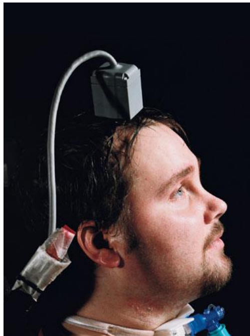
Fig. 1c: Braingate, an example of invasive BCI based on intracortical recordings
