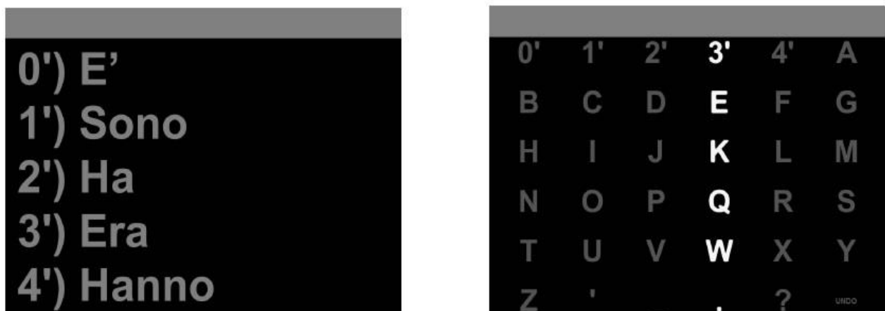
Fig. 2.2a: an example of selection operated with the Polymorph system. On the left, suggestion that user can examine before starting character selection. On the right, the panel for item selection: in their first row symbols 0', 1', 2', 3' and 4' allow to directly write words suggested in the previous phase
