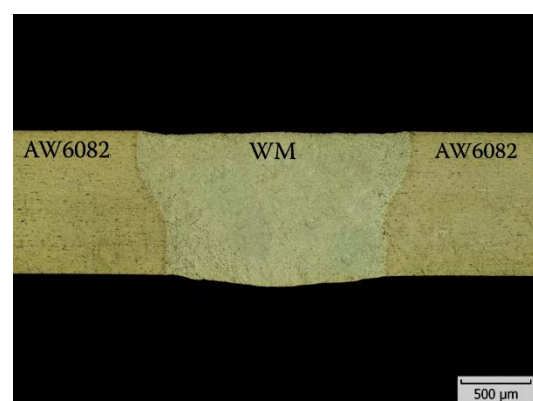
Fig. 1. Cross section of selected weld joint
