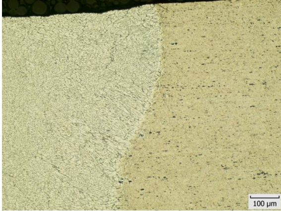
Fig. 2. Weld metal – AW6082 interface
