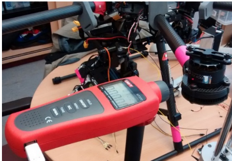
Fig. 2. Measuring the angular velocity of the motors.
