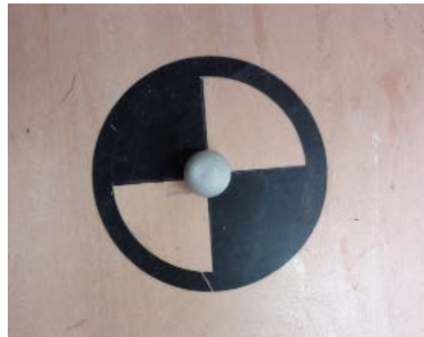
Fig. 1. IR marker placed on the geodetic reference point.
