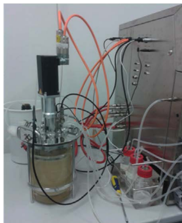
Fig. 4: bioreactor Biostat B, (Sartorius) assembled with a 2L vessel, and parameters used to express Pin1.
